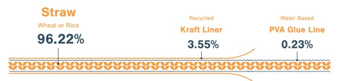
Durra Panel can be used on its own as a wall and ceiling lining or be combined with Durra Steel Sections to form a wide range of panelised roof, ceiling and wall systems with an extensive track record over 70 years for use in commercial, industrial and residential projects. Durra Panel has been successfully used in project applications such as airports, stadiums, schools, industrial facilities and homes.
