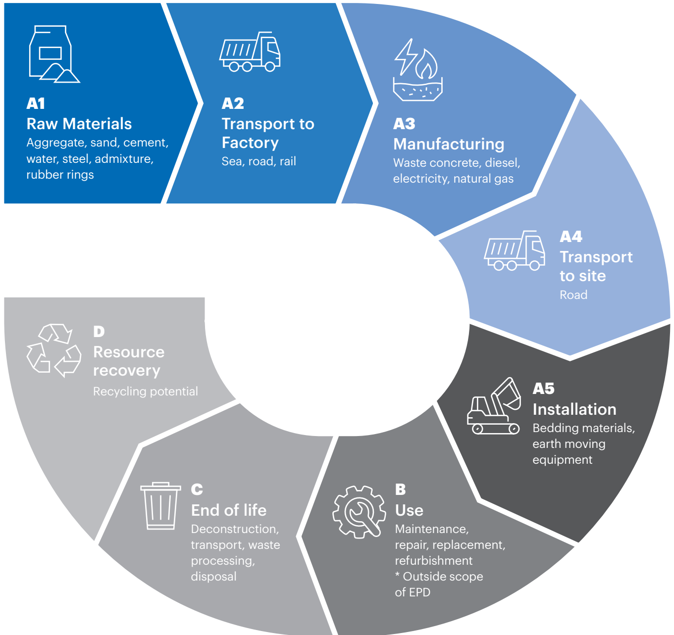
Figure 1 – Product lifecycle of steel reinforced pipes
