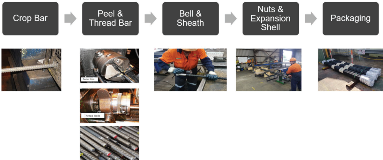
Figure 2: Manufacturing Process of CT Bolt
